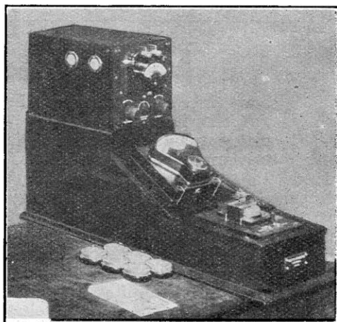
The test set employed for determining the sensitivity of receivers. The principle of operation of this set is shown diagrammatically on the next page.
