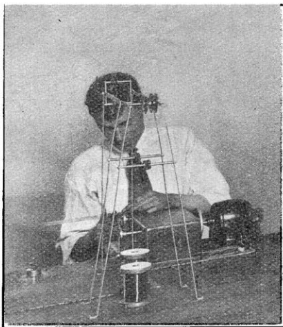
Winding the bobbins. The machine automatically counts the turns run on, and trips when the winding is completed.
